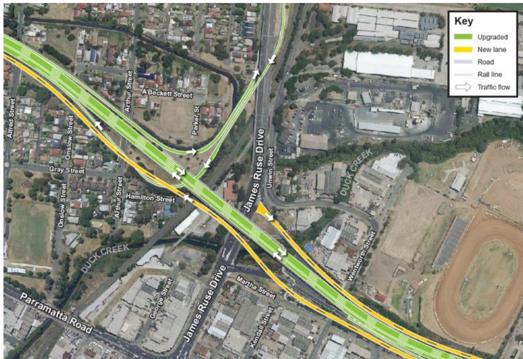
Figure 3.2 WestConnex upgrade at James Ruse Drive – widening and new ramp configuration
